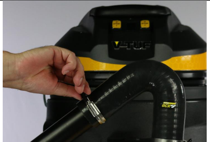
Tighten Thumb Screw 2(Nm).
