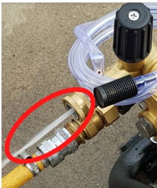
Fig3: High pressure outlet: This is where the high-pressure hose connects.
