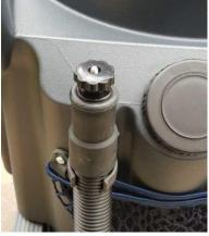
The vacuum has a float valve to seal the air flow to the vacuum motors when the liquid being vacuumed reaches the maximum level in the tank.
