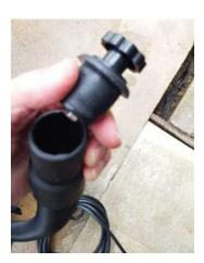
3. Drop drainpipe to an area you wish to dispose if the liquid. (See below) Please note: You cannot run the vacuum motors while doing this.
