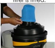
Ensure the head is correctly fitted and the clips secure. For dry, non- hazardous material, ensure the HEPA filter is fitted.
